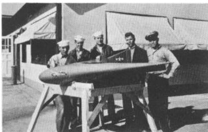
One of the BuAer projects at Annapolis was a radio-controlled flying wing. This particular version made one successful free flight, dropped from plane.
